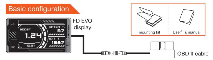
● FD EVO uses standard CANBUS communication, connecting to OBD II for full vehicle scanning and quickly displaying 22 driving data points from the ECU.
